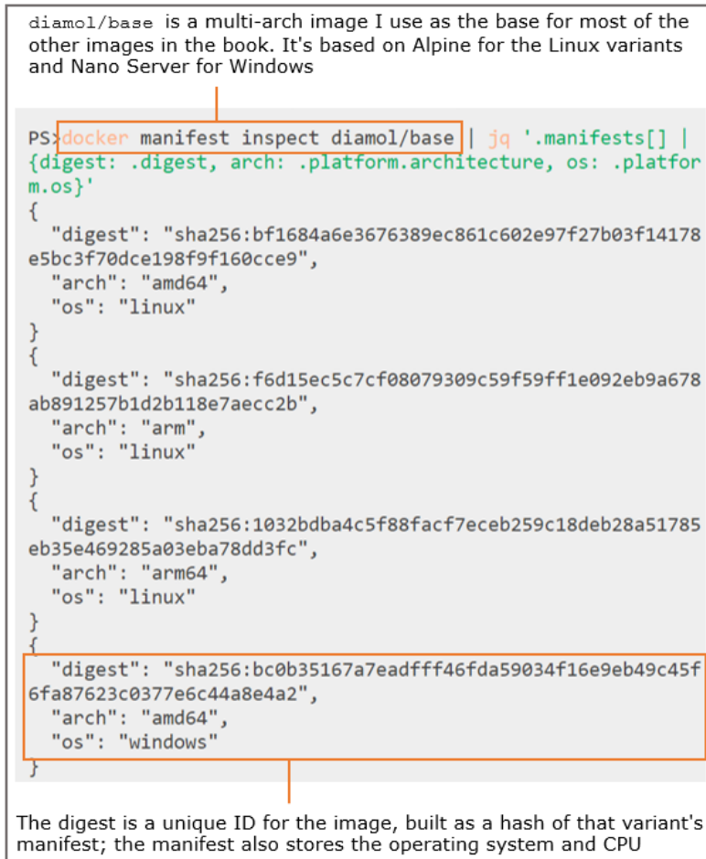
Figure 16.10 Multi-arch images have several manifests; each contains the architecture of the image
