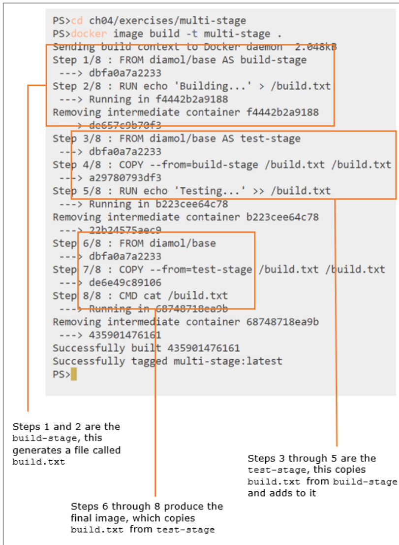
Figure 4.3 Building a multi-stage Dockerfile
