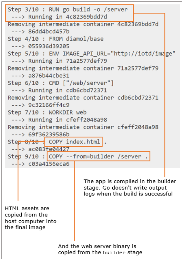
Figure 4.9 Building a Go application in a multi-stage Dockerfile
