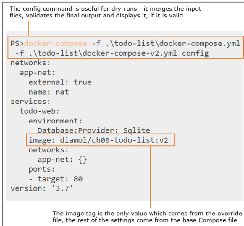
Figure 10.5 Merging a Compose file with an override file and displaying the output
