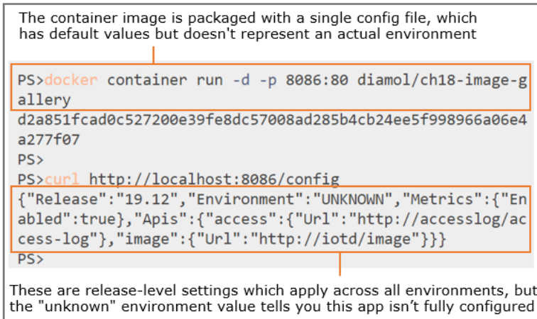
Figure 18.7 You can package your app with default settings which work but aren't a complete environment
