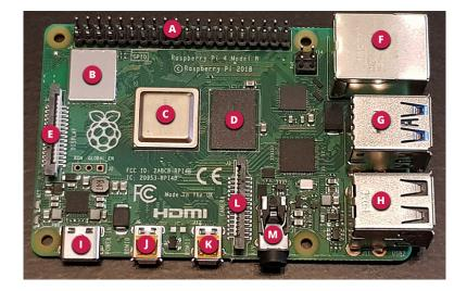
Here are the main components of the Raspberry Pi 4:
