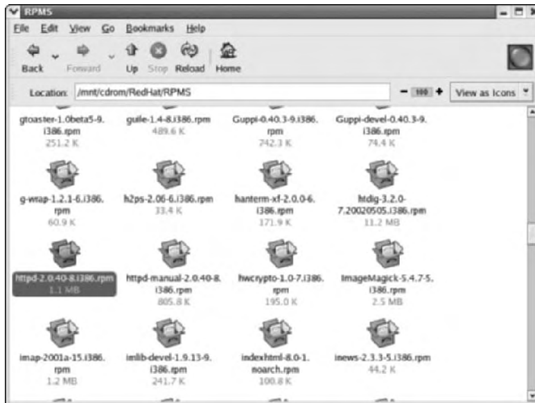
Figure 1-7 You can install a package by finding it with a file manager (such as Nautilus, pictured) and double-clicking the file name.
