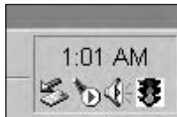
Figure 3-8 When hidden, WinMySQLAdmin displays a stoplight icon in the task bar. Click the icon and choose Show Me to redisplay the graphical interface.
