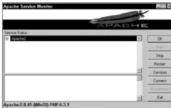
Figure 2-4 You can control the Apache server with the Apache Service Monitor.
