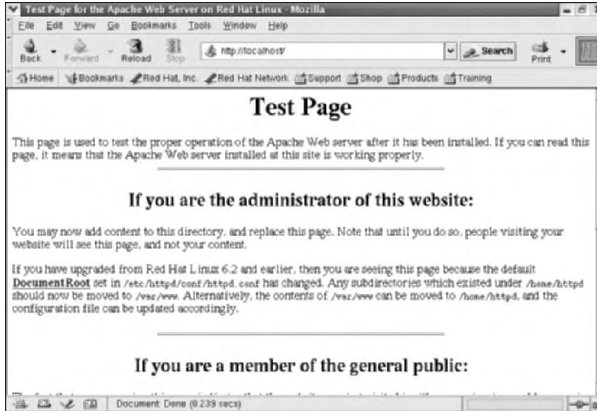
Figure 1-9 The Apache test page confirms that the server is up and running.
