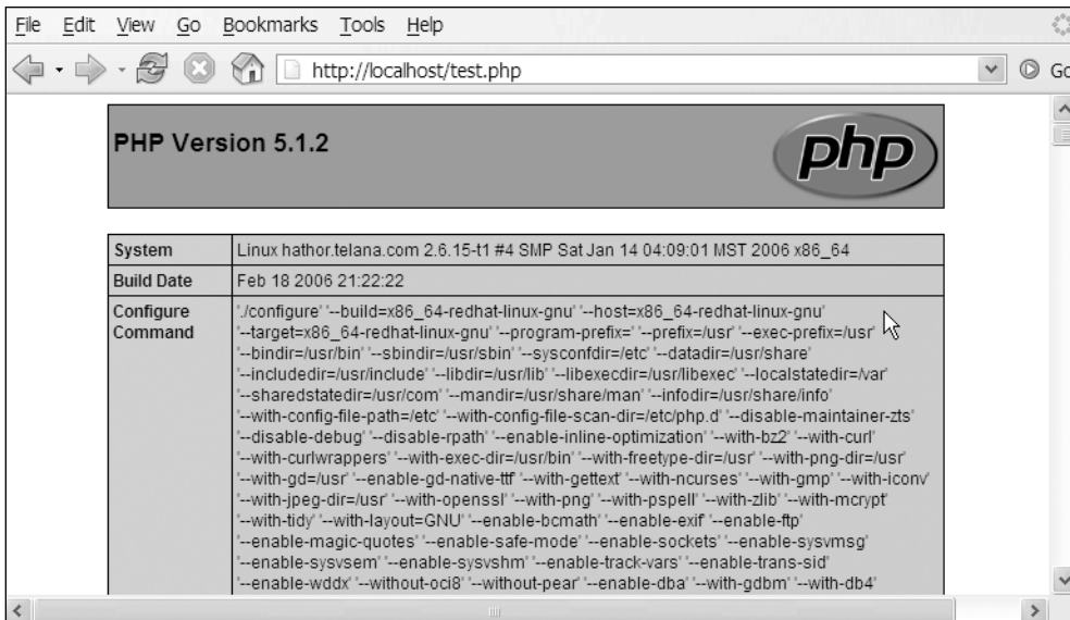
Figure 3-5. The browser displaying the phpinfo() output confirming that Apache and PHP are installed correctly
