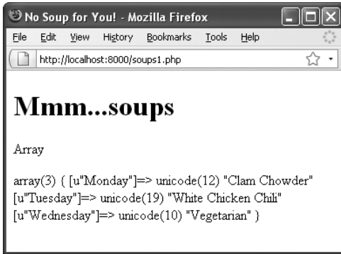
Figure 7.2 The var_dump() function (used with Script 7.1 instead of the print_r() function) shows how many elements are in an array and how long each string value is.
