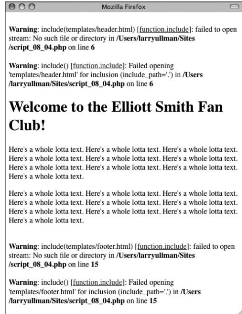
Figure 8.7 When an include() fails, warnings are issued, but the script continues to execute.
