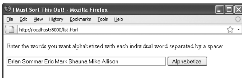
Figure 7.9 This HTML form takes a list of words, which is then alphabetized by the handle_list.php script (Figure 7.10).
