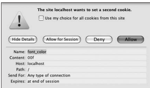
Figure 9.7 The second cookie that's sent is called font_color and has a value of 00f , representing the color blue.
