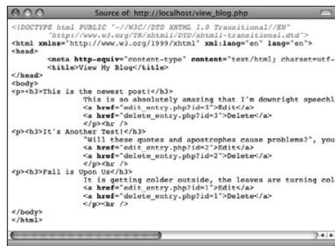
Figure 12.20 Part of the HTML source of the page. Note that the two links have ?id=X appended to each URL.
