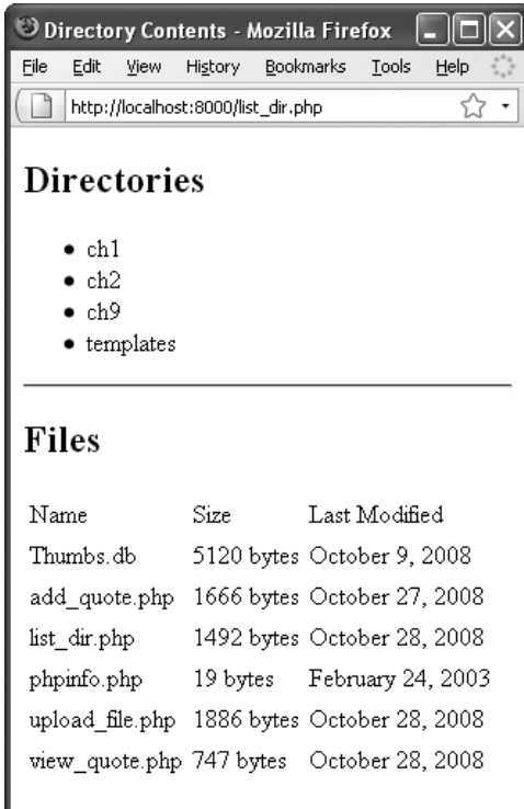
Figure 11.21 The list_dir.php script shows the contents of a directory. The top part lists the subfolders, and the bottom table lists the files.
