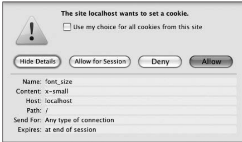
Figure 9.6 The user sees this message when the first setcookie() call is made, if they've opted to be prompted before accepting a cookie. This cookie is storing the value of x-small in a cookie named font_size .
