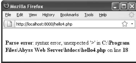
Figure B.4 Parse errors are all too common and prevent scripts from executing.
