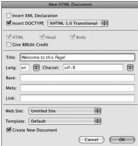
Figure 1.1 BBEdit and most other Web development applications will create the basics of an XHTML document for you.
