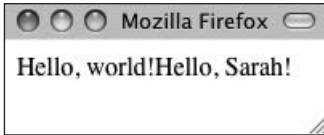
Figure 10.5 Calling the function without any arguments uses the default value (the first greeting); calling it with an argument provided means that value will be used instead (the second).
