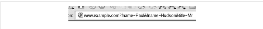
Figure 9-2. HTTP GET sends data in the URL in a very obvious manner
