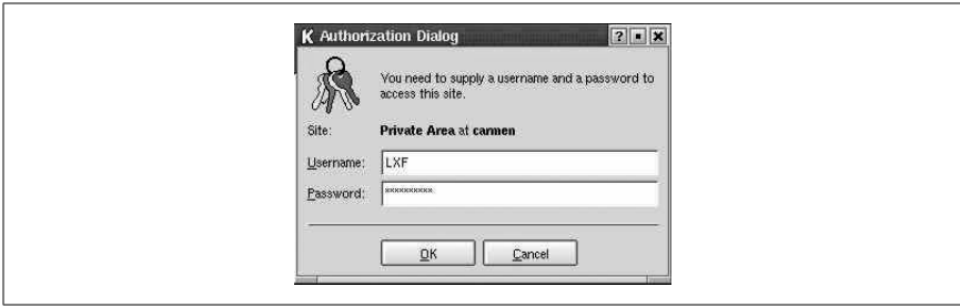
Figure 20-2. HTTP authentication is a simple way to keep parts of your site safe from prying eyes
