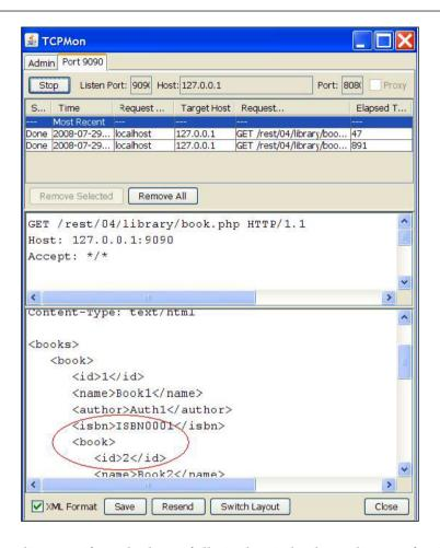
In the above diagram, if you look carefully in the circle, the ending tag for the book element is missing. A new starting tag for a new book is started before the first book is closed. This would cause the XML parsing on the client side to fail. In this case I am using the Library system sample and here is the PHP source code causing the problem.
