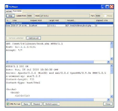
As you can see, the tool has captured the request and the response. The request appears at the top and the response at the bottom. The request is a GET request to the resource located at /rest/04/library/book.php. The response is a success response, with HTTP 200 OK code. And after the HTTP headers, the response body, which is in XML follows.
